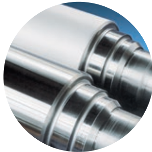
The matt surface of the skin pass roller shows the TOPOCROM® coating.
